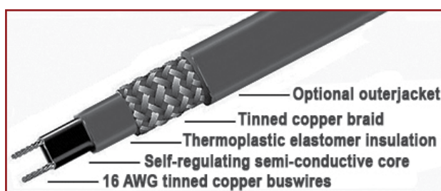
Cutaway view of ProLine self-regulating heat cable.
